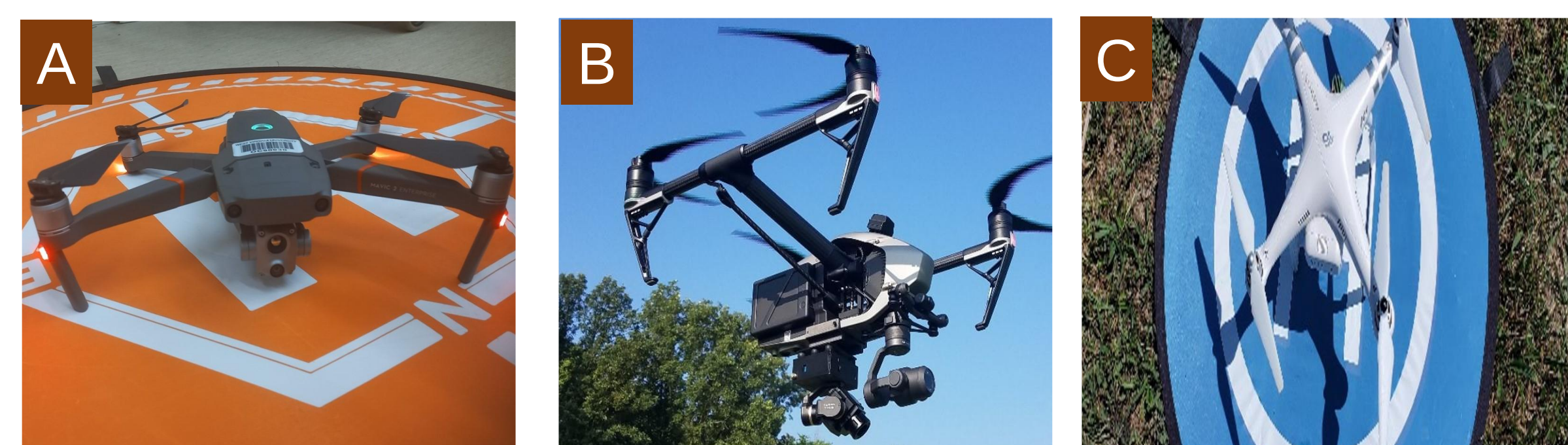
Fig. 1. Drones used for this study: Mavic Enterprise Advanced with Thermal and RGB sensors (A), and DJI Inspire 2 with NIR and RGB sensors (B), and Phantom 3 with NDVI and RGB sensors (C)
